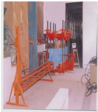
Fig. 1: The system to pullout the shaft placed to form holes for pre-perforation
