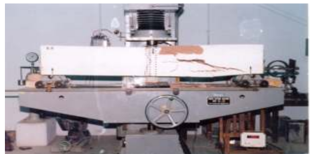
Fig. 9: Pre-compression baked clay beam is testing on Torsion Testing Machine
